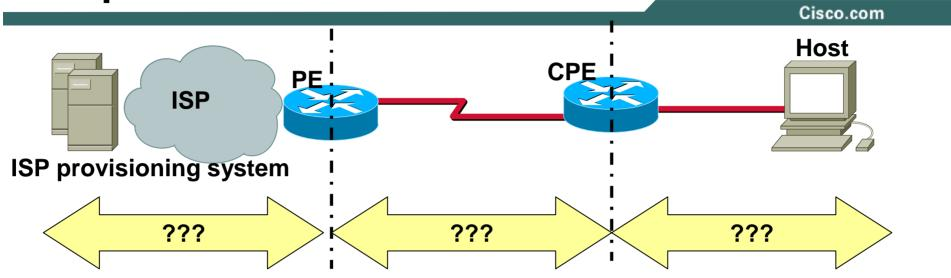
How do we get the configuration information and prefixes from the ISP provisioning system, to the PE, from the PE to the user CPE, and from the CPE to the end user hosts?
